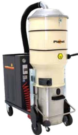
**PLANET 775 ATEX** CE EX II 3D Ex t III B T135°C Dc IP55
