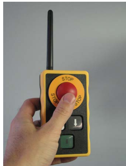
Emergency Stop- Remote Control Panel
